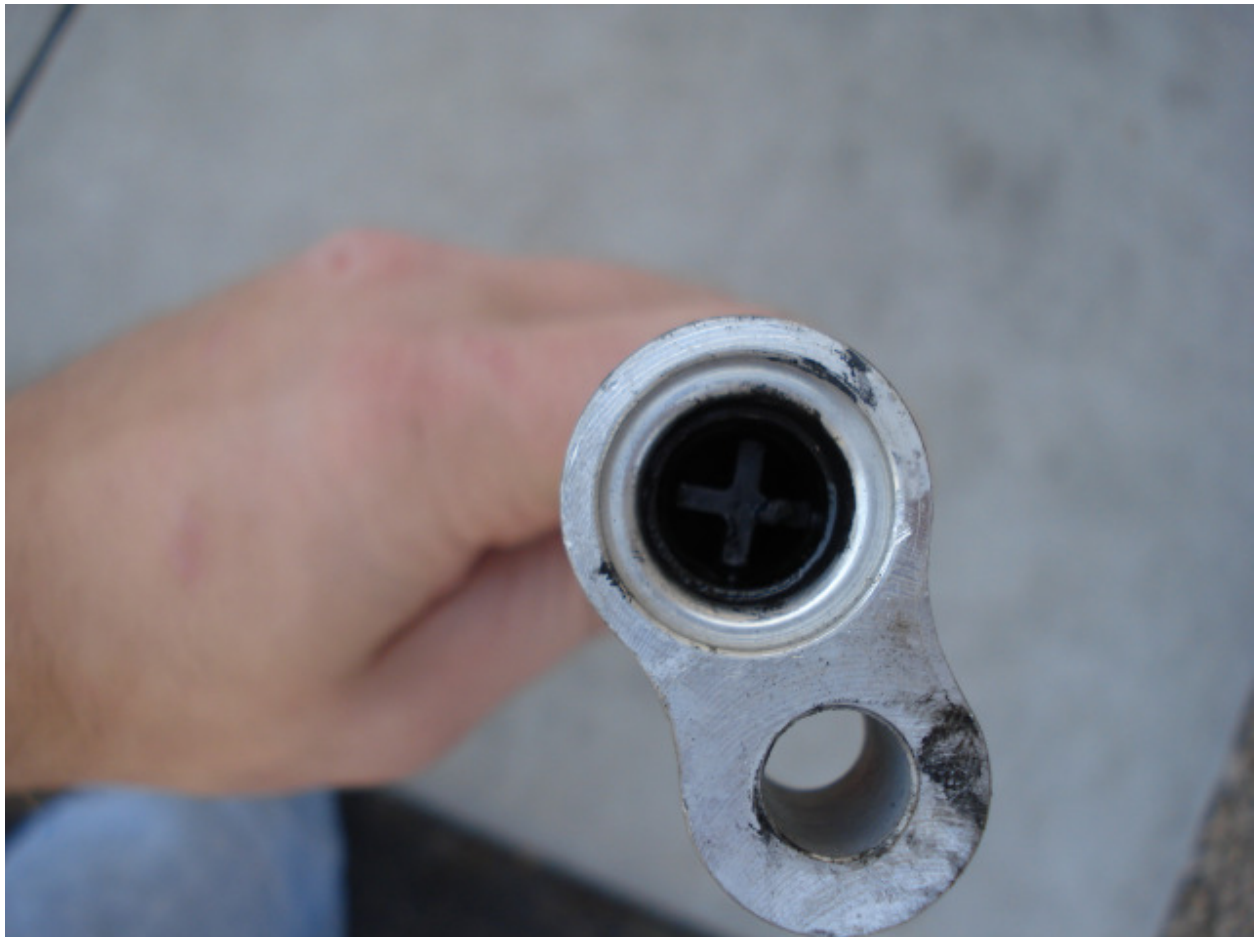
looking at the orifice tube in the line:
